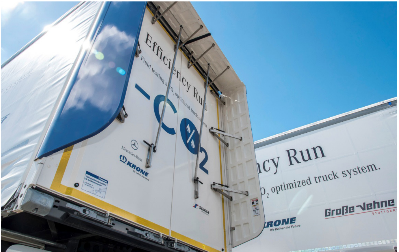
Figure 9: Application of rear flaps (source: Daimler Efficiency Run)
