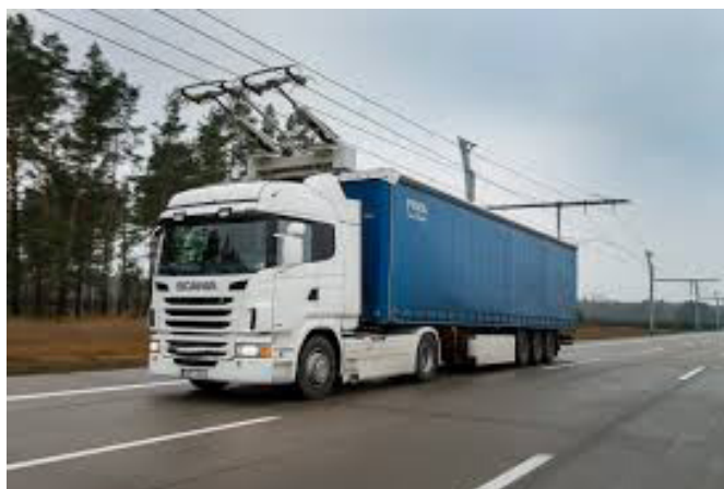
Figure 5: ERS in operation (Source: Scania)
