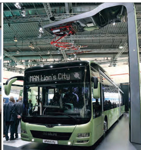
MAN Lion's City eMobility is a concept of electric city modular bus with numerous combinations of batteries and electric engines packs depending on the operator's needs, production of which will start in 2020
