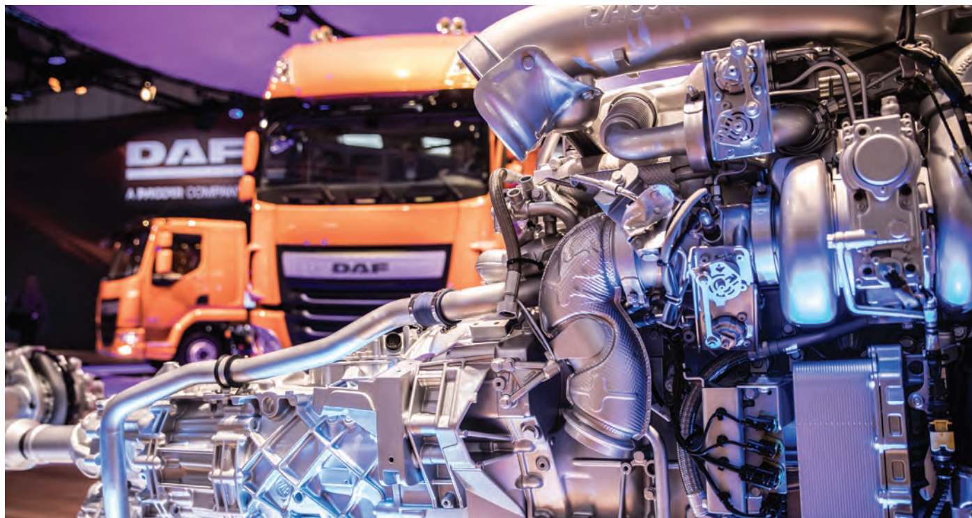
DAF has provided instruction of what we will encounter in the new XF generation. The exhibited prototype is a test platform with diesel-electric hybrid drive, which mainly uses the energy generated for propelling the ancillary system, and it will be capable to pass the last 3 to 5 kilometres before reaching the destination with zero emission
