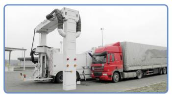
The other type of scanner moves along the vehicle. The driver exits the vehicle and waits outside the exclusion zone.
