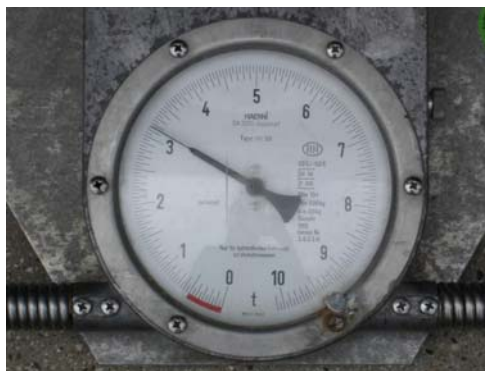
Figure 2.3 Portable analogue vehicle weighing equipment in Austria
