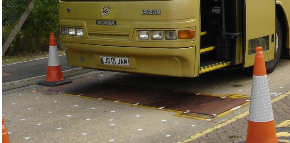
Figure 2.4 Permanent digital vehicle weighing tool United Kingdom
