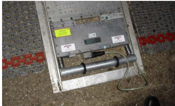
Figure 2.2 Portable digital vehicle weighing equipment in the Netherlands
