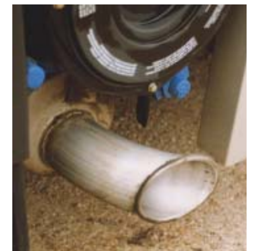
CRT filtre which reduces hydrocarbon and particle emissions by 80-90%
