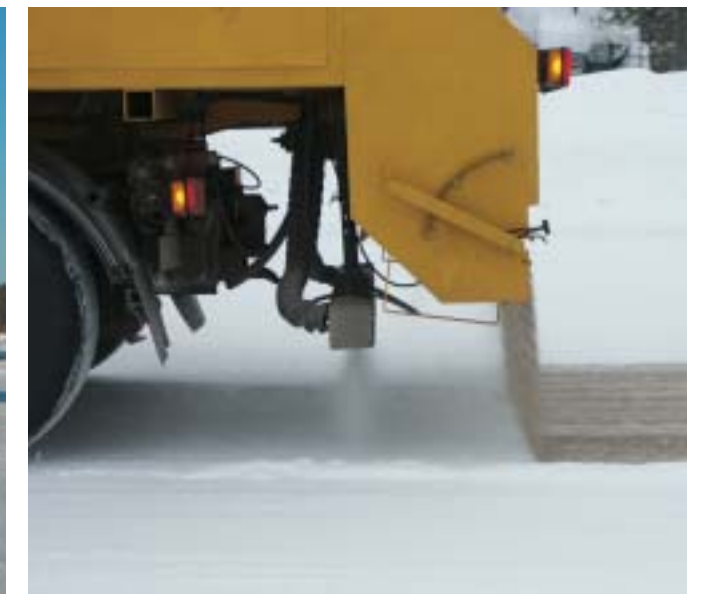
Moist grit being launched via a rotating disc
